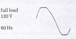
Waveform peaks clipped at 90° by pulsating current flow. Average responding voltmeter reads too high. Peak responding voltmeter reads correctly.
