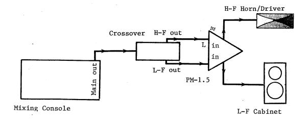
The diagram shows the connections for such a system. Here, the high-frequency output of the crossover is connected to the left-channel input of the PM-1.5, and the low-frequency output of the crossover is connected to the right-channel input. Connections are made between the respective loudspeaker elements and the amplifier's output terminals. Of course, the loudspeakers in this set-up, like any dual-channel set-up, must have a nominal impedance of  $4\Omega$  or greater.
