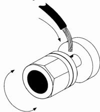
Figure 8. Bare Wire Connection
