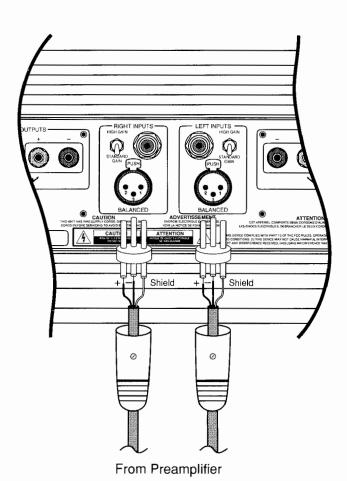
Figure 7. Balanced Input Connection
