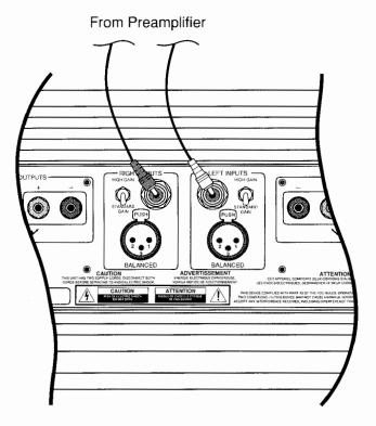
Figure 6. RCA Input Connection
