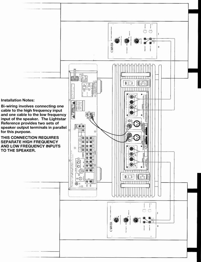
Figure 4. Bi-Wired Connection to Speakers with built-in crossover
