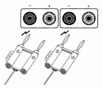
Figure 10. Banana Plug Connection
